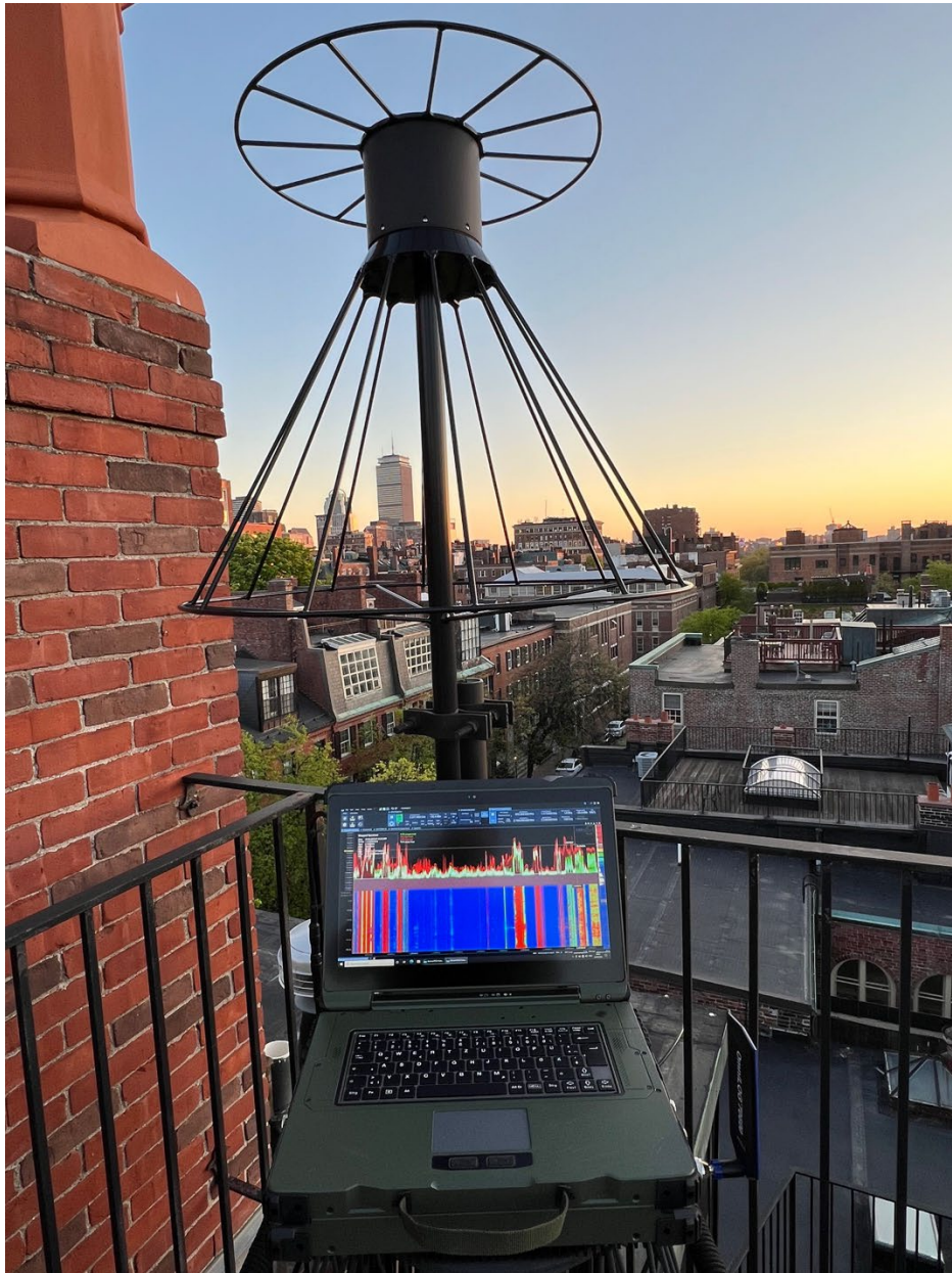
Figure 1: A spectrum analyzer allows engineers to visualize the RF spectrum. Equipment like this reveals complex interference relationships between seemingly unrelated wireless networks.
