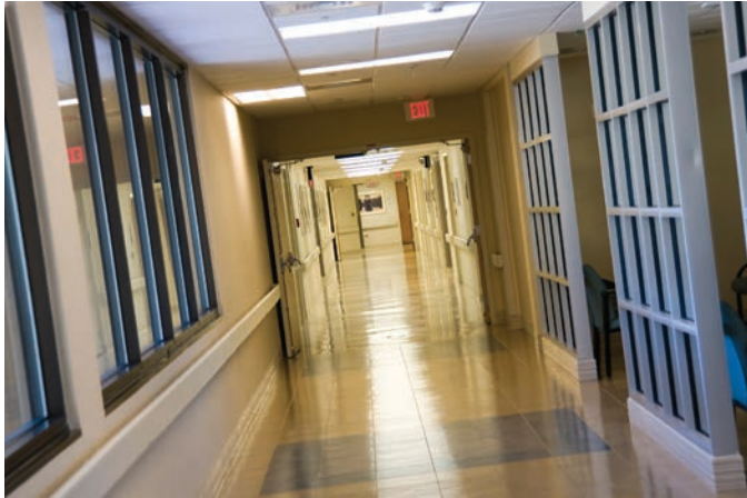
Hospital compartments must have travel distances of no more than 200 feet to reach another smoke compartment.
